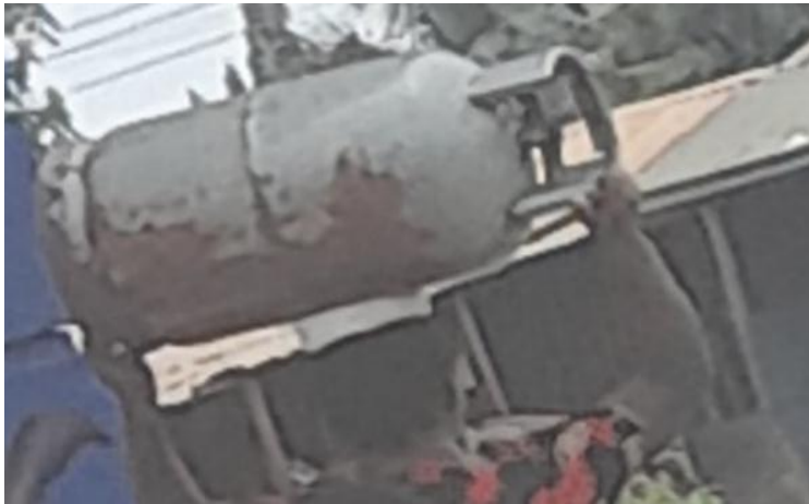
Figure 8 (c): A Filled Rusted Cylinder Carried Horizontally
