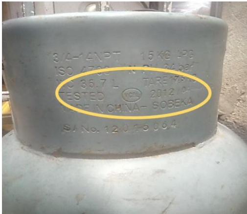
Figure 5: An Expired Mandatory Test Date for an Imported LPG Cylinder
