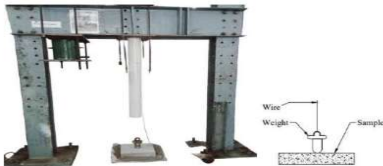
Figure 9: Diagram Illustrating the Drop-Weight Test Setup
