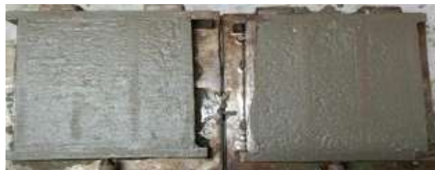
Figure 6: Casting and Curing of Specimen for Flexural Test
