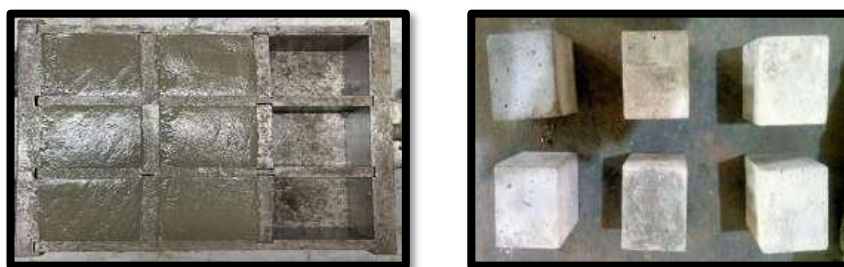
Figure 3: Curing and Casting of Cubes for Compression Test
