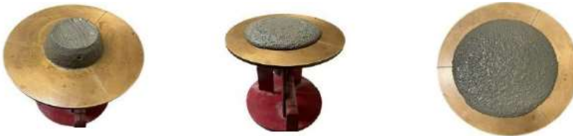
Figure 10: Laboratory Arrangement or Setup for Flowability Test
