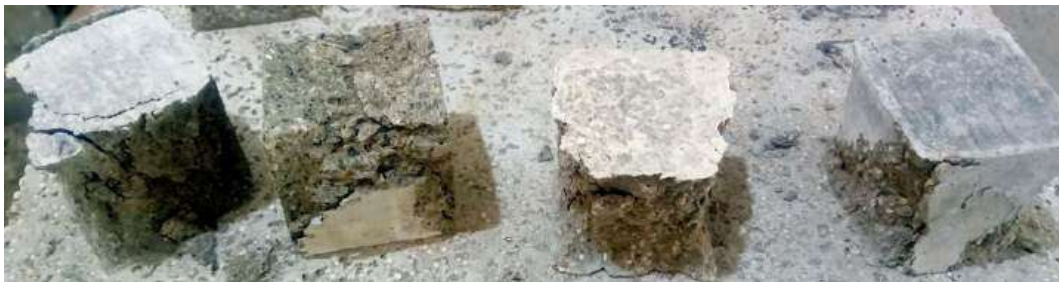
Figure 12: Specimens after Compression Test
