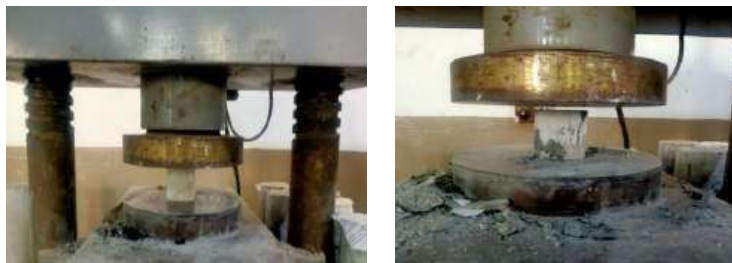
Figure 5: Laboratory Setup for Compressive Strength Test
